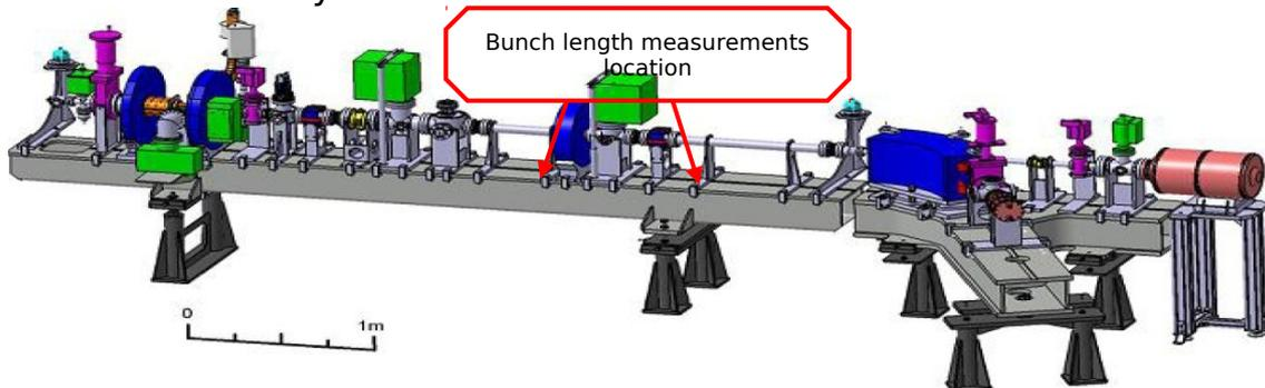
Fig.3: A drawing of the beamline on PHIL
