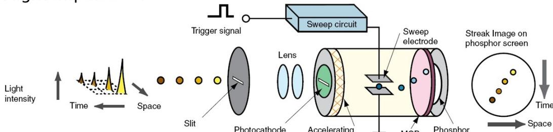
Fig.1: Operating principle of the streak camera
