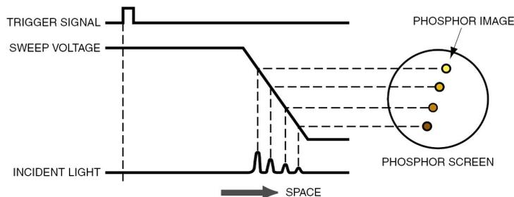
Fig.2: Operating timing principle
